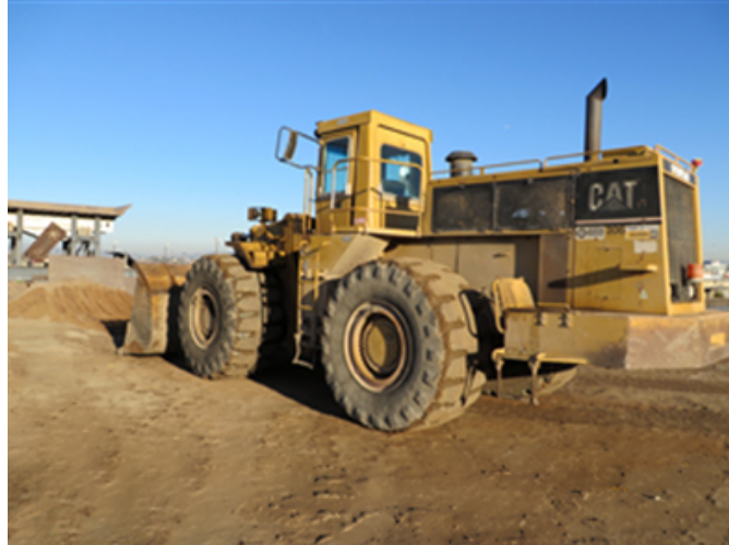
Concrete Crusher loading hopper (left) & Tier 3 engine Rubber Tire Loader (center)
