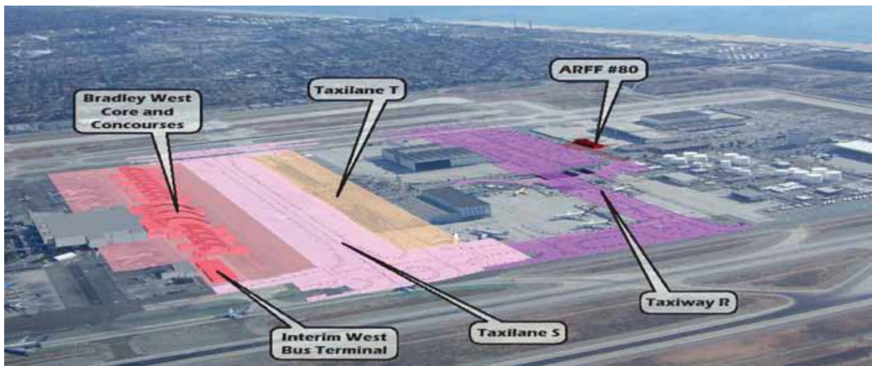
Figure 1.2.1-1: Taxiway T Phase 1 Construction Location on the Airfield
