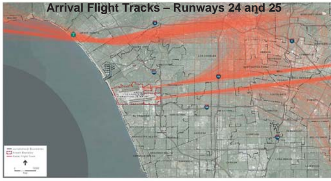
Los Angeles International Airport - 14 CFR Part 150 Noise Radar Flight Tracks - Arrivals from the East Exhibit C-1 Los Angeles World Airports
